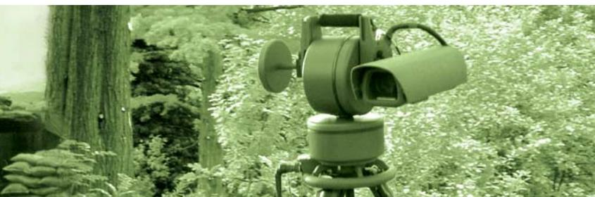
*PIVOT (Pillar Versatile Observation Turret) is a rapidly deployable and man-portable surveillance system. It consists of a high-speed pan-and-tilt turret equipped with a Day Dawn Camera driven by a Control Unit with a high-resolution and high-brightness LCD screen.*
